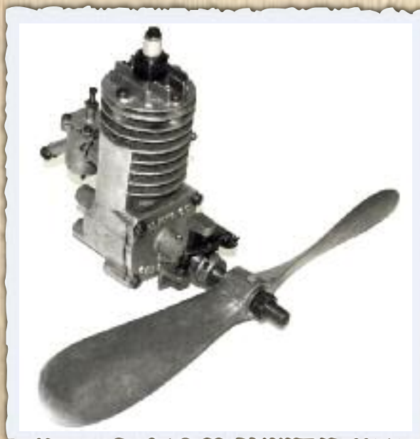
A 1922 Gil Aero Midget 1.18 cid with its factory-installed 12-inch aluminum propeller.
