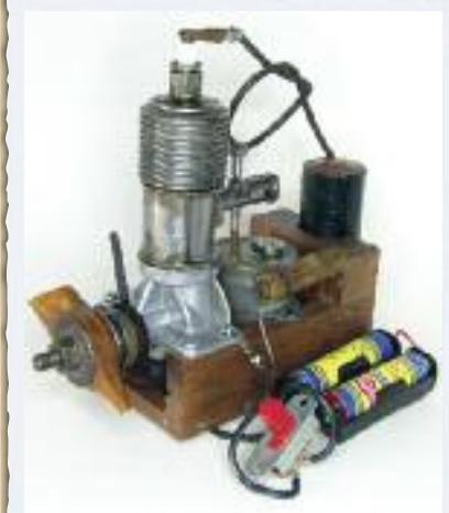
The 1937 Junior Motors Brown B .60 cid, was nearly identical to the 1934 model, with coil, condenser, and batteries. All had to be carried aloft!
